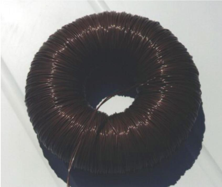
This sensor contains about 2000 turns of the #20 AWG enameled wire and has a total dc resistance of 7.4 Ohms. I estimate that it took about 8 hours of winding to create this sensor – done a bit at a time while watching TV in the evenings or while having morning coffee.
