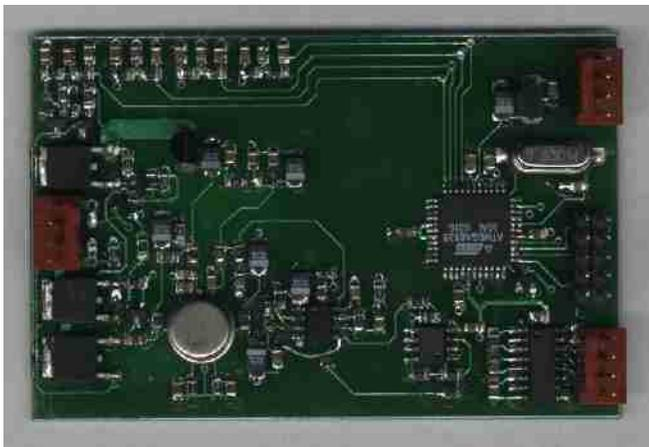
very approximately 5cm by 8 cm in size and uses mainly surface-mount components. The brown connector on the left side connects to the sensor. The top connector on the right side connects to the battery and the lower one is the RS-232 interface to the outside world. The program allows one to set parameters like the polarization time, number of
